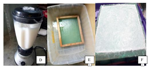
Figure 4: Sheet making process; D = Pulp blending, E = pulp pouring, F = Sheet draining
